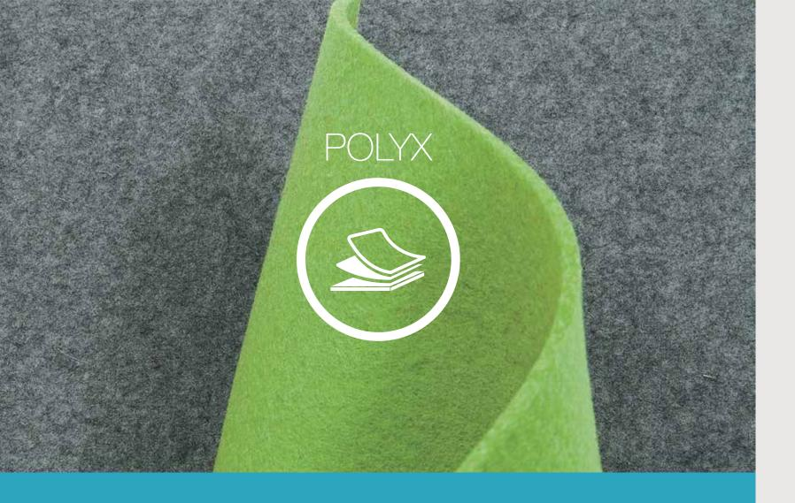
POLYX Polyester Board is made by a process of tumbling, needle-punching, and baking low and high melting-point polyester fibres. The high-density fibrous network absorbs sounds and reduces reverberation. POLYX Polyester Felt is made with only high melting-point polyester fibres, which gives a softer touch and a vibrant colour. The Polyester Felt can be laminated on top of the Polyester Board.
